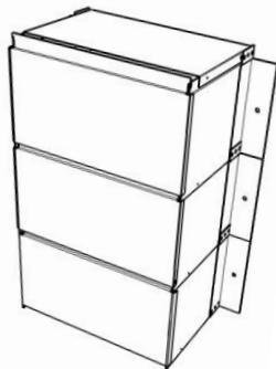
Empty Battery Box
