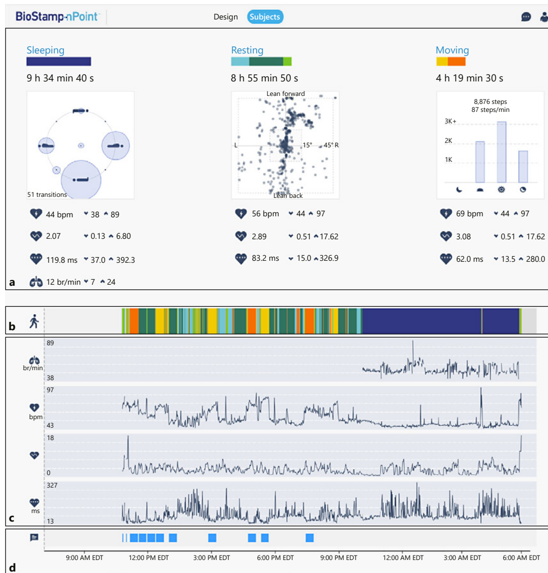
Fig. 1. Investigator portal dashboard displaying representative examples of participant data from one day of wear including daily summary outputs associated with sleeping, resting, and moving activities (a), longitudinal view of color-coded actigraphy during sensor wear (b), RR, HR, HRV ratio, and HRV RMSSD during sleep (c), and instances of annotated study activities (d). Graphs for HR, HRV ratio, and HRV RMSSD are auto-scaled for display purposes and for representing data for an approximate 24-h recording. HR, heart rate; HRV, heart rate variability; RMSSD, root mean square of successive differences; RR, respiration rate.
