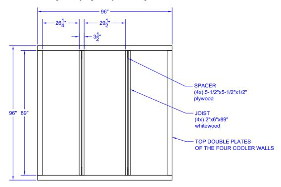
• Make two double ceiling joists by nailing together two 89 inches long white wood 2 by 6 boards with two pieces of 5-1/2" x 5-1/2" x 1/2" thick plywood spacers – one spacer on each end.
