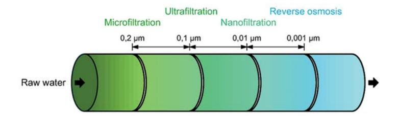
Membrane based water treatment uses varying sizes of membranes to filter out contaminants from water based products or waste streams using mechanical separation. Membrane technology can also be combined with other treatment methods when contaminants cannot be filtered out.
