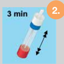
2. Extraction is done by shaking the tube for 3 min
