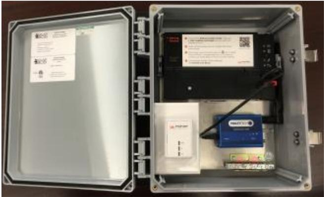
**Attabox AH12106 Enclosure with BP1210A back plate**
