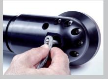
The bottom of the furler unit has a point for attaching a Dyneema® bobstay
