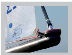
The LOOP® EF1500 is mounted on a J70 Gennaker pole
