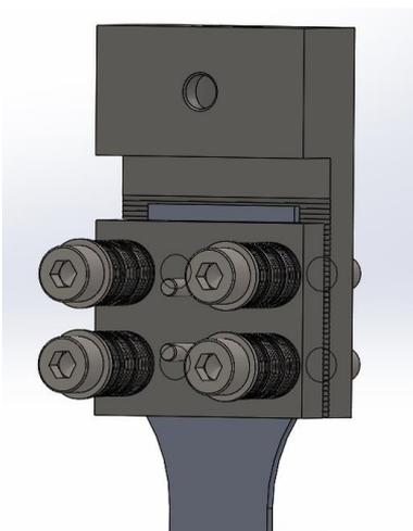
**Fig. 2:** Grip design to avoid slipping
