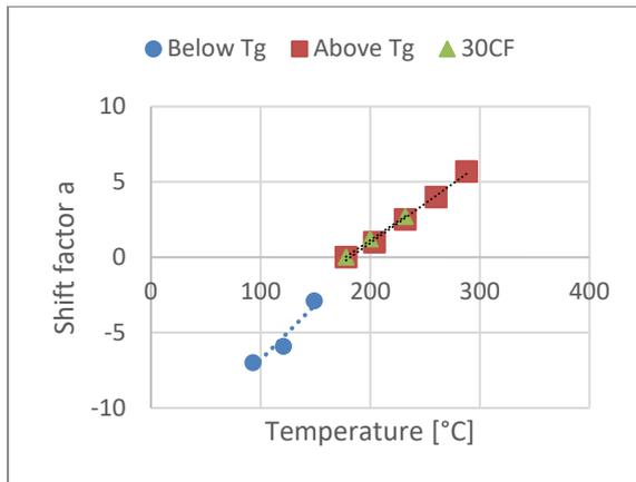
Fig. 5: Shift factor to obtain the master curve
