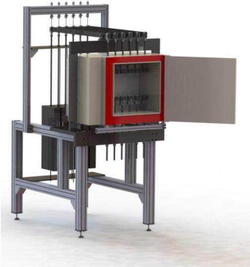
**Fig. 1:** Creep testing jig with 6 positions
