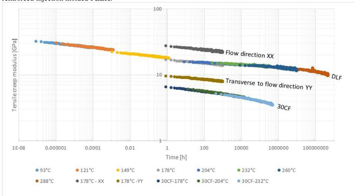
Fig. 6: Mastercurve of DLF. For comparison we added High flow DLF in flow and transverse to flow direction as well as 30% short carbon fiber filled PEEK. The data is shifted to the reference temperature of 178°C using time-temperature-superposition.
