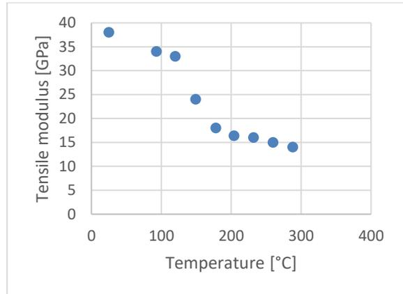
**Fig. 3:** Instantaneous modulus as a function of temperature
