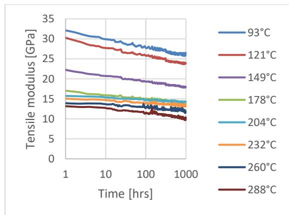
**Fig. 4:** Creep modulus for DLF at various temperatures
