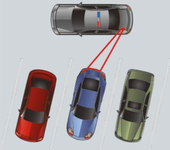
**ELSAG ALPR cameras can scan license plates on vehicles in perpendicular and angled spaces**
