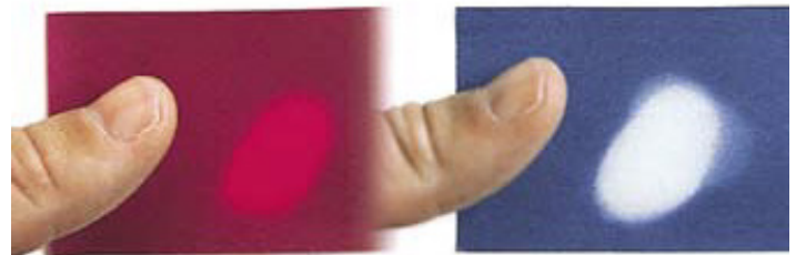
THERMOCHROMIC SPECIMEN DISPLAYING INK CHANGING TO COLORLESS STATE AND ANOTHER COLOR UPON HEAT-ACTIVATION BY RUBBING FINGERS TOGETHER
