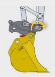
c. Lift the dipper arm until the coupler is completely disengaged from the attachment pin. The attachment is now disengaged. Deactivate the power button by pushing power
