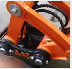
17. Run 2x mm hose up dipper arm, using mm hose clamps to secure them in place as shown in photo
