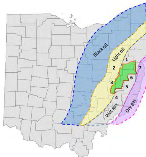
Figure 1: Outline map of Ohio State showing the location of the 3D seismic survey used in the study. The numbers 1 to 7 show the individual counties discussed in the text over which the 3D seismic survey was shot. Overlaid on the outline are the different hydrocarbon phase windows, showing that the survey falls in the wet gas/light oil window. The data for the hydrocarbon phase ribbons was adapted from Mariani (2013).
