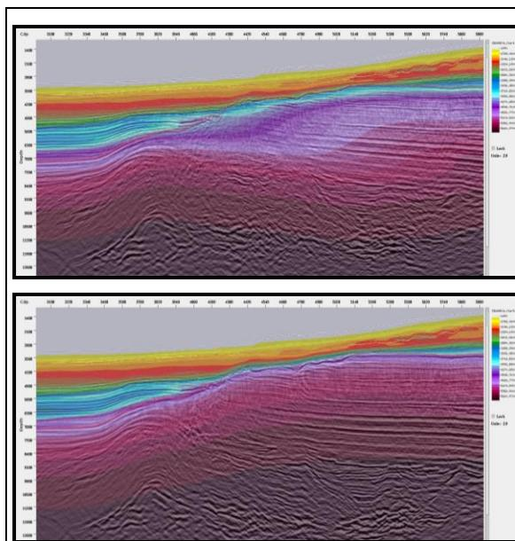
Figure 4: Before (top) and after (bottom) inserting fast velocity below the Aptian unconformity, the velocities are overlaid on a stack. The Jurassic carbonate events are well-focused and continuous.
