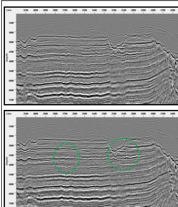
Figure 6: Before (top) and after (bottom) the horizon-constrained tomography to reduce the undulations of Jurassic carbonate. The tomography reduced the undulations, which are not geologically plausible.
