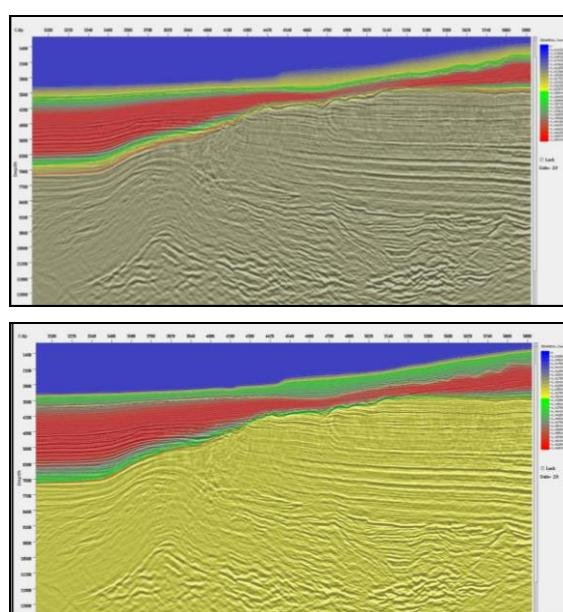
Figure 2: Anisotropic parameters, delta (top) and epsilon (bottom), as a color overlay on a Kirchhoff PSDM stack.
