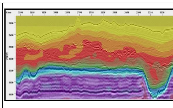
Figure 8: The complex geology above the Aptian unconformity. The high resolution tomography update captures the local velocity anomalies. However, FWI can produce a more detailed velocity.
