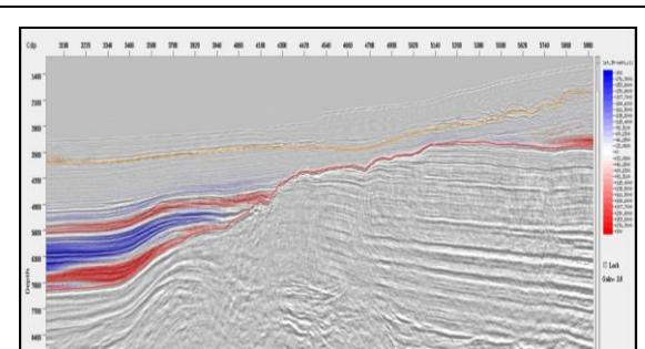
Figure 3: The tomographic update (DV) is overlaid on a stack. Image guided tomography provides the updates along the geological structure.
