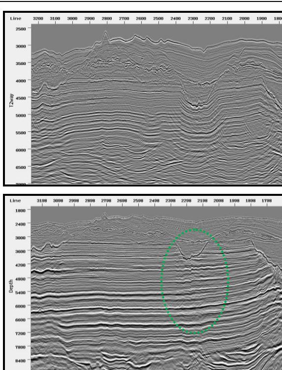
Figure 7: PSTM (top) vs PSDM (bottom). The carbonate layers are well imaged and truncated to the unconformity in PSDM.
