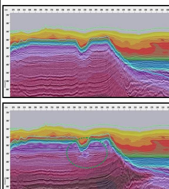
Figure 5: Before (top) and after (bottom) the high-resolution tomography. The event continuity is enhanced and the relatively high frequency undulations are reduced.
