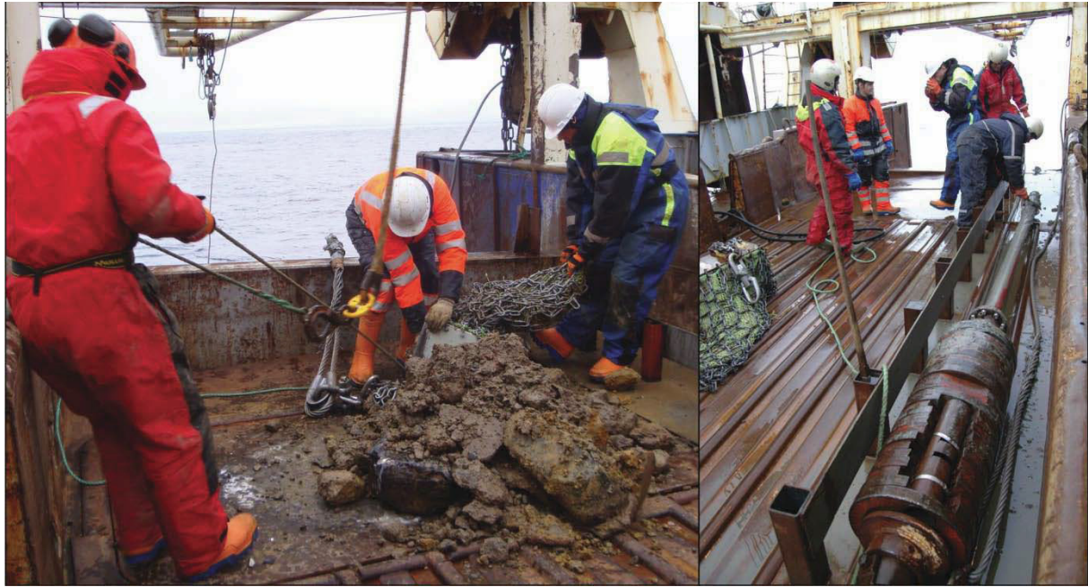
Figure 2 Left: Contents of a dredge emptied on the deck. The hemipelagic clay is washed and rock fragments arranged in lithological groups. Right: Gravity corer recovered on deck, the cutting shoe is removed and checked for the presence of hydrocarbons. The liner is then extracted from the core barrel, cut into 1 m sections, and sampled.
