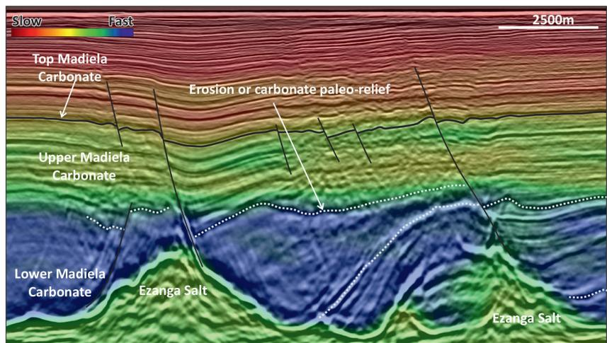
**Figure 3** Seismic overlay of the Final Velocity Field with Kirchhoff PreSDM in depth. The velocity field allows characterizing different facies within the Madiela Carbonate. The stratified limestones of the upper section are slower and potentially more rich of siliciclastic deposits. The lower section shows seismic velocities up to 6000 m/s and is dominated by massive carbonate and dolomites (Lower Madiela).
