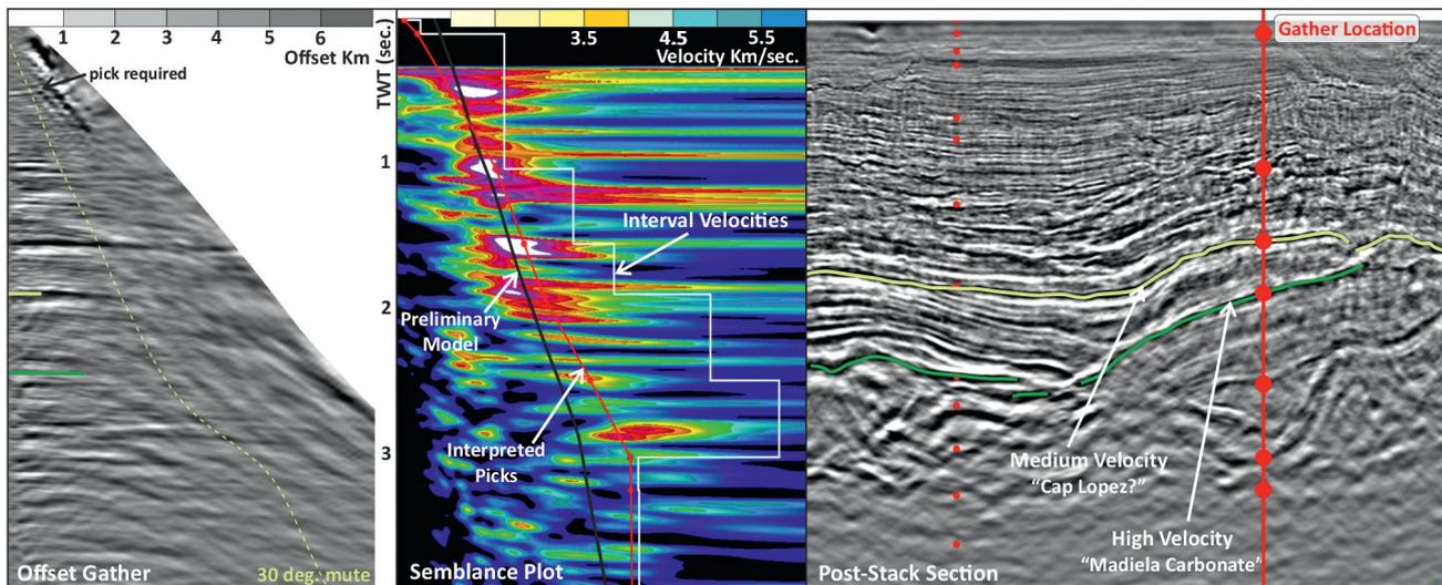
**Figure 5** Gather picks obtained from the interpretation of the main velocity breaks.
