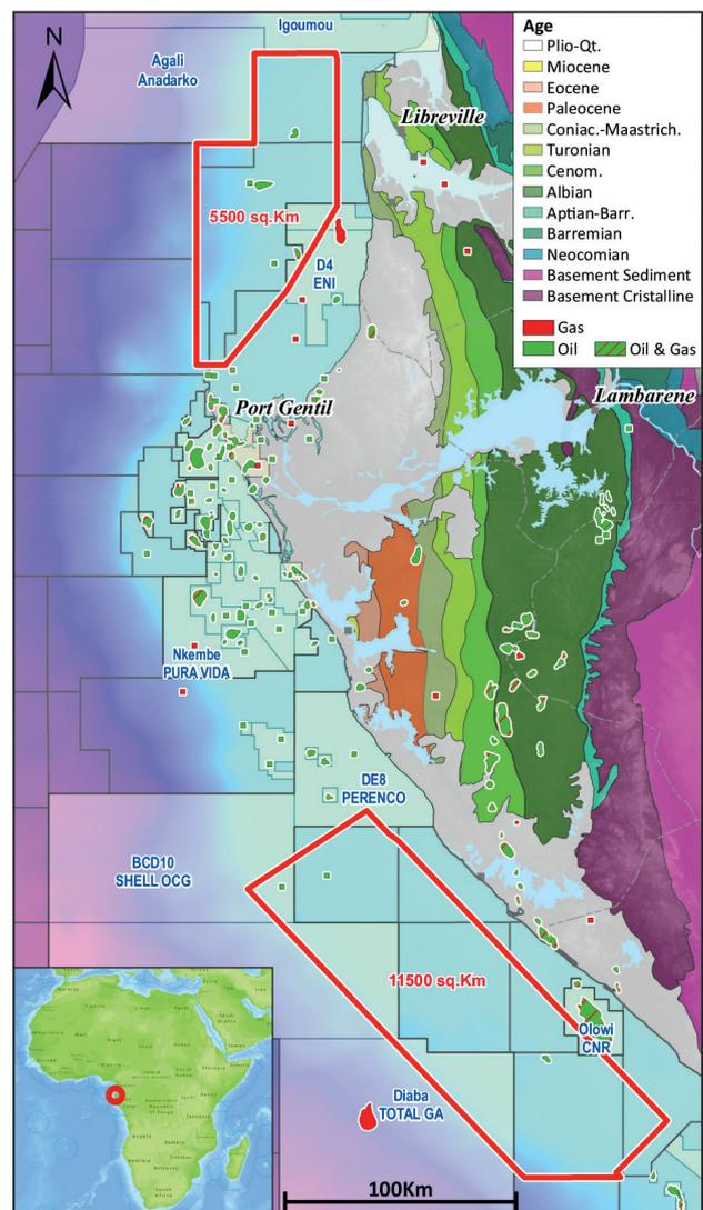
Figure 1 Map showing the Spectrum's Multiclient 3D seismic surveys offshore Gabon. Onshore geological map in the background (Thomas et al., 2001).
