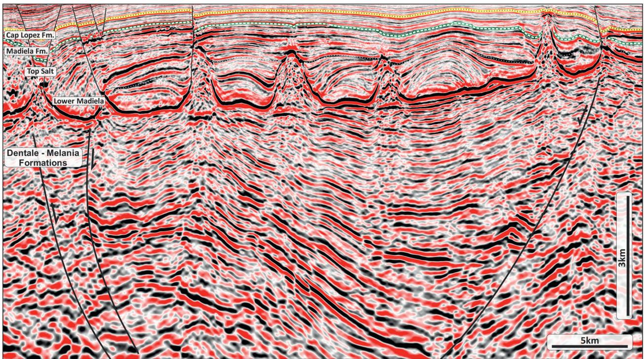
**Figure 2** Depth seismic profile extracted from the southern 3D survey. The section is obtained by an algebraic combination of the final RTM (Reverse Time Migration to 30 Hz) with near and middle angle stacks from the Kirchhoff PreSDM. (The same final velocity model was used in both migration algorithms.)
