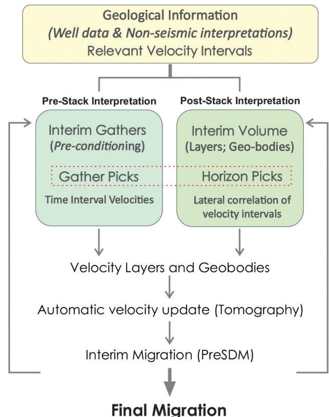
Figure 4 Simplified workflow for pre- and post- stack interpretation.
