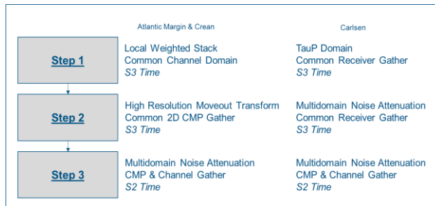
Figure 4. Schematic representations on deblending workflows for the three surveys.
