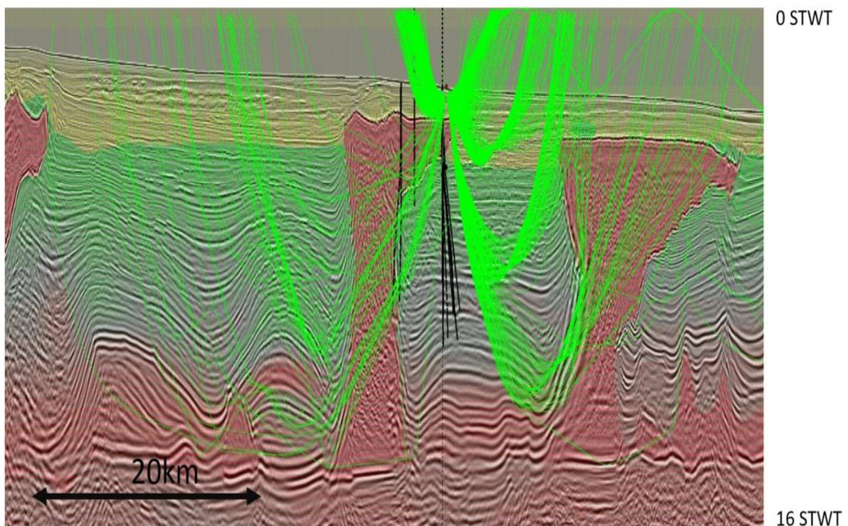
**Figure 1** Ray trace Modelling, showing shots shooting into a single subsurface recorder.
