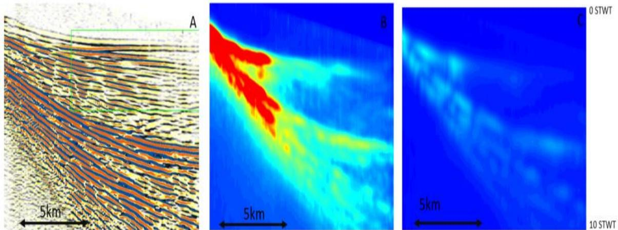
**Figure 3** A) Receiver gathers from single shot line with linear move out of 3350 m/s. B) Receiver gather amplitude envelope below 15 Hz. C) Receiver gather amplitude envelope below 5 Hz.
