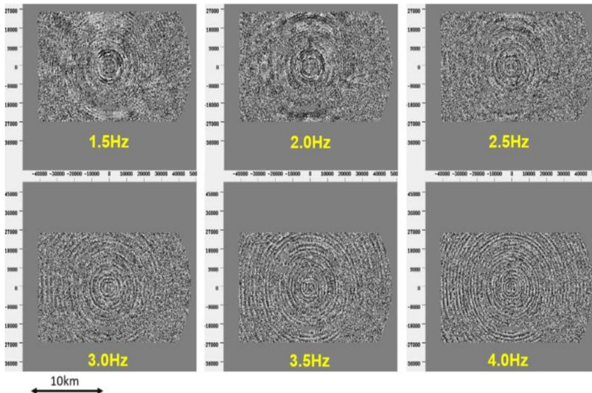
**Figure 4** Phase ring plots of receiver gathers from a 2950 cubic inch air gun, it can be observed that the frequencies below 3 Hz are visible approximately 3 km before disappearing in the noise floor. Above 3 Hz there is good continuity of the signal to the observed 8 km offsets.
