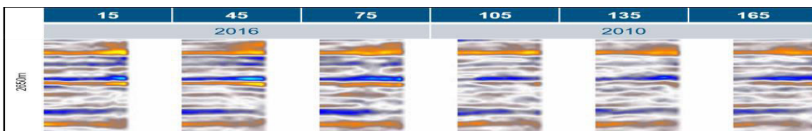
Figure 6 Example of production-induced change in signal on azimuth. Overall, the gathers are identical in the 6 azimuths except the event at 2650 m, where there is a correlation between the acquisition year. The first three azimuths are from 2016, the second three azimuths are from 2010.
