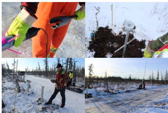
Figure 3: Custom sensor cup at end of loading pole with 3C analog geophone and sandpoint. Orientation tool. Recording equipment connected and QC'd. Planting tool in action.
