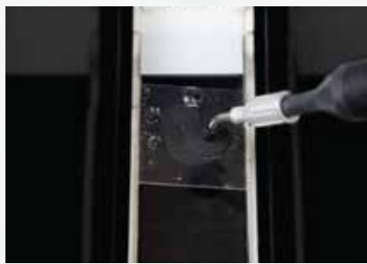
Place coverslip to make micro-chamber
