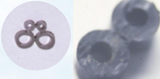
Plastic tubing has a very large surface area to volume ratio. It also is a source of carbon for Bacteria. The hydrophobic surface makes biofilm attachment easy. Some tubings have a rough interior as they are extrusion molded.
