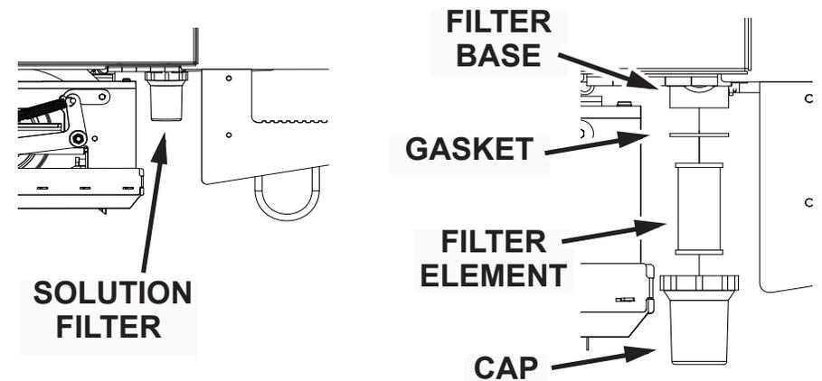
Fig. 2: Water Solution Filter with Exploded view
