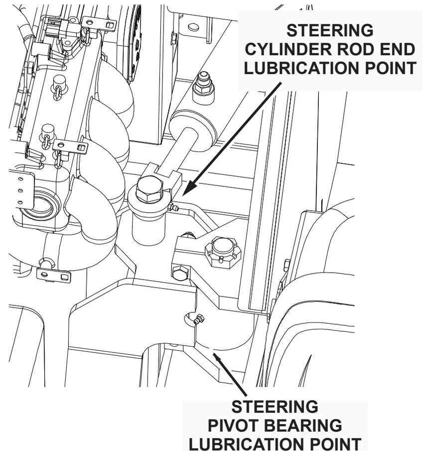
Fig. 1: Lubrication Points
