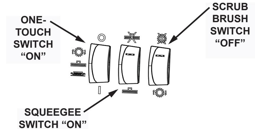
Fig. 1: Control Settings for Water Pick-up Mode
