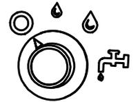
The **Low flow setting** is for normal scrubbing, smooth floors, and light dirt. The flow rate is .88 gal/hr (3,33 L/hr), providing 2.0 hours of scrub time.
