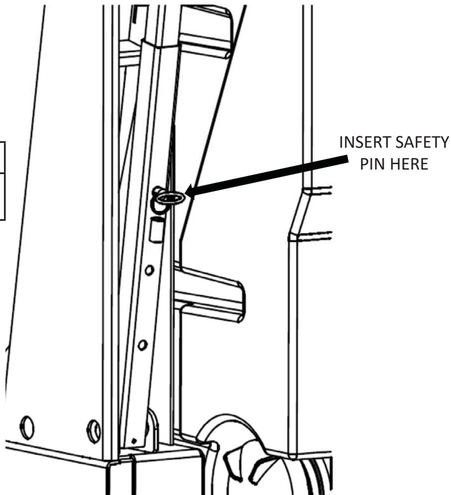
3. Remove the hopper lift safety pin from the back of the left side support tube.
