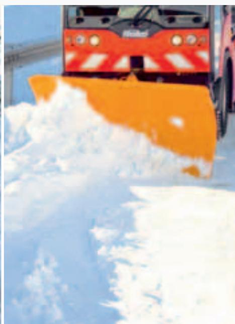
A front-mounted sweeper (160 cm), various snow blades (working width up to 170 cm) and a spreader mounted to the rear coupling triangle allow for fast and easy snow clearing without demounting the hopper.
