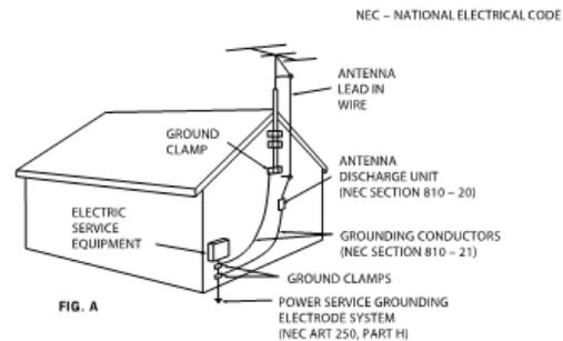
NOTE: This reminder is provided to call the CATV system installer's attention to article 820-40 of the NEC that provides guidelines for proper grounding and, in particular, specifies that the cable ground shall be connected to the grounding system of the building, as close to the point of cable entry as practical.
