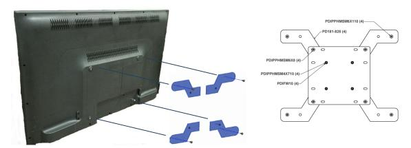
ATTACH THE PD181-672 PLATE (#1) TO THE EXISTING 100mm VESA MOUNT USING FOUR PDIPPHMSM4X76 SCREWS (#4) AND FOUR PDIITLW10 WASHERS (#3). MAKE SURE THE EXISTING MOUNTING BRACKET IS ATTACHED TO THE SIDE OF THE CHOSEN PLATE WITH THE FOUR ROUND ENDS OF THE M4 INSETS. THE SIDE WITH THE FOUR HEX ENDS WILL GO TOWARDS THE BACK OF THE SET.
