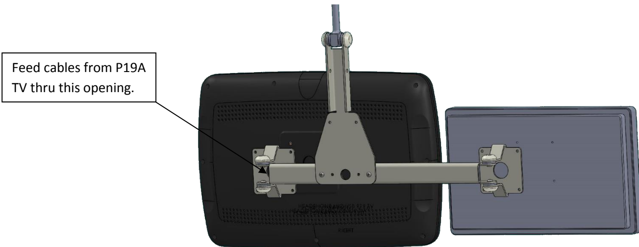
FIGURE 3. CONNECTING THE DUAL MOUNT ARM
