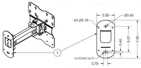
STEP 3: Insert PD181-839 (#4) bracket to PD181-707 (#1) mount by carefully aligning PDINILN1032 (#5) nut through the keyhole on the main plate of PD181-707 mount. Finally, tighten PDINILN1032 (#5) nuts on both the top and the bottom adaptor bracket PD181-839 (#4).
