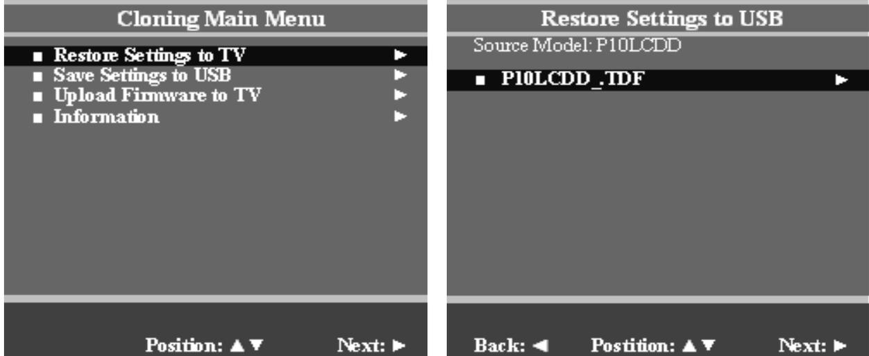
3. Press ▲ OR ▼ to select Restore Settings to TV. Press ► to display a list of previously stored TV setups on the USB thumb drive.
