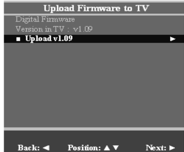
13. Press the ▲ direction button in the Automatic Upload Firmware to TV menu to begin uploading the new firmware. Or, in Upload Firmware to TV, press ▲ or ▼ to highlight the desired version of firmware. Then press ▶ in the Upload Firmware to TV menu to begin uploading the new firmware.
