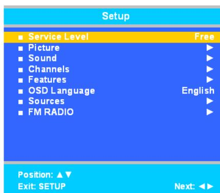
**Disabled** is like a mechanical key lock – when in *Disabled* service level, the TV can be turned OFF and ON, but cannot be used for viewing. A standard message appears on a black screen.
