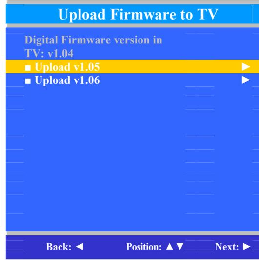
14. Press the ▲ direction button in the Automatic Upload Firmware to TV menu to begin uploading the latest firmware. Or, in Upload Firmware to TV, press ▲ or ▼ to highlight the desired version of firmware. Then press ► in the Upload Firmware to TV menu to begin uploading the new firmware.
