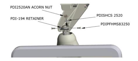
5. Close the nose cover of the arm and securely reattach the PDIFHMS83250 screws.
