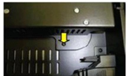
7. Connect the other end of the cable to one of the connectors on the side of the TV. Tighten with the thumb screws on both sides of the cable.
