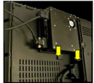
5. Line up the screw hole on the module with the screw hole that is just above the vents.
