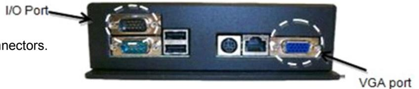
4. Slide the computer module into the top position so the ports are facing the outer edge of the side of the TV.
