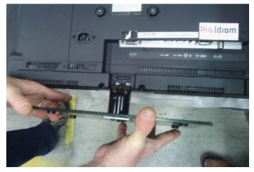
3. Place stem of stand into bottom of TV and using drill, secure with 2 supplied screws as shown.
