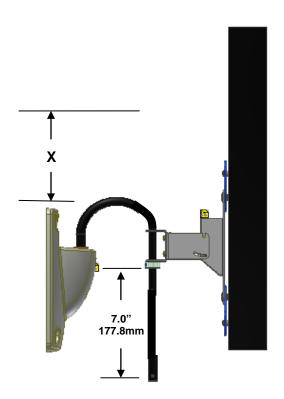
X - Varies on the placement of the wall bracket and the size of TV
