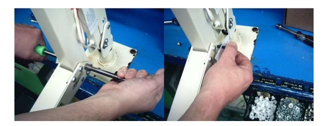
Loosen brakes: back off the brake tension screws about ½ a turn
