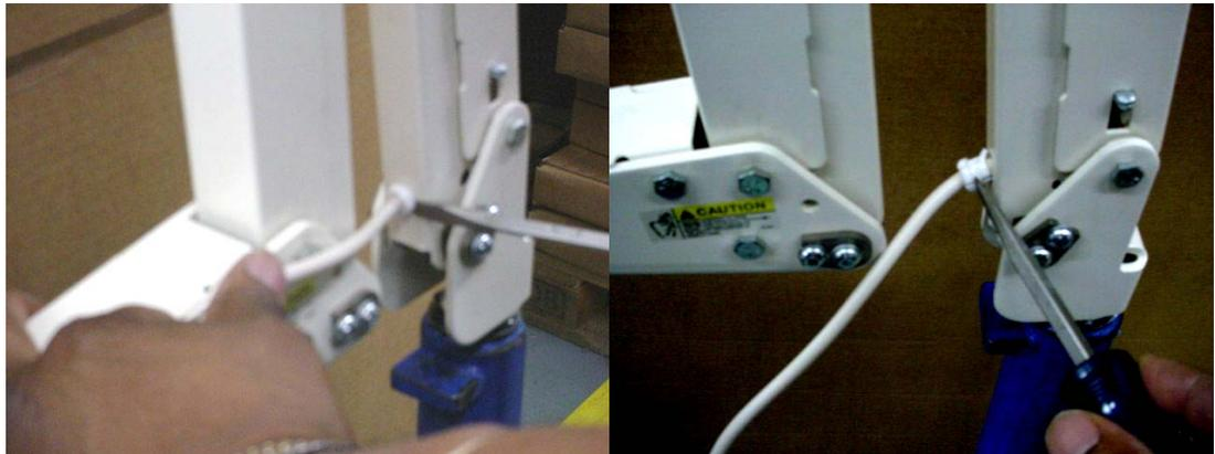
4. Cut off the connector and pull the damaged cable through the back of the arm.
