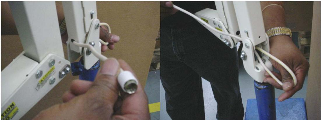
5. Pull the cable through the elbow section.
