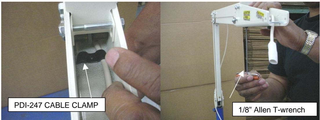
7. After removing the PDI-247 cable clamp remove the damaged cable.
