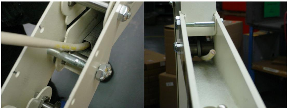
8. Cable Obstruction Note: Push cable through the wire-shield, when there is a cable obstruction at the braking system, Push down slightly on the nose and twist and push cable until the cable goes past.(see open arm Illustration )
