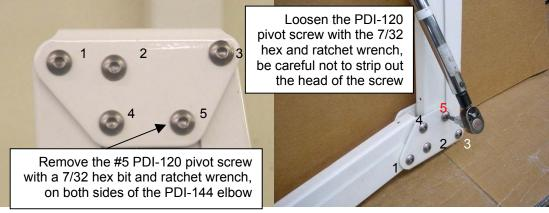
• Next lay the arm on the bench and remove the screws
