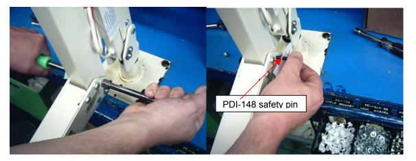
• Move the arm into the up position, remove the PDI-247 cable clamp in the nose with the 1/8" T-wrench., turn t-wrench counter clockwise to loosen.
