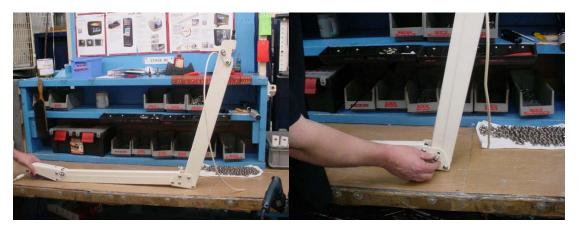
• Next lay the back section down and pull out the damaged cable.
