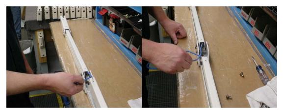
• After cable is completely out of the back section, pull it out of the front section
