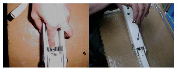
• Re-assemble back arm section with PDI-120 pivot screws, and apply a drop of red 271 loc-tite to the threads of each screw. Torque each screw to 17-1/2 foot lb.s
