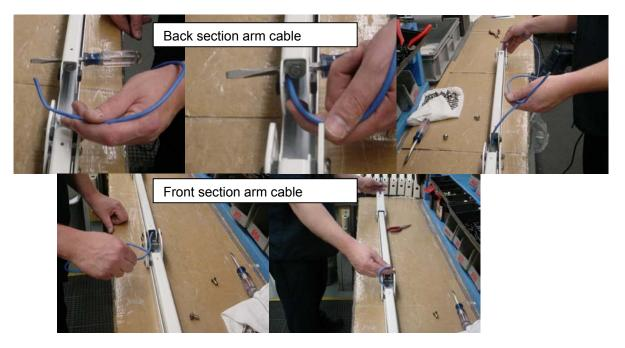
• Cable Obstruction Note: Push cable through the wire-shield, when there is a cable obstruction at the braking system, Push down slightly on the nose and twist and push cable until the cable goes past.(see open arm Illustration )
