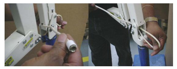
• Cut off the connector and pull the damaged cable through the back of the arm.
