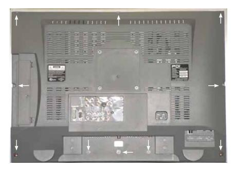
3. Now remove the EMI shield by first removing the eight screws, which secure the shield with a P2 screwdriver. Note which screw secures the Ground Wire. Be CAREFUL not to harm the wire harness or yourself with the sharp edges of the shield during removal.
