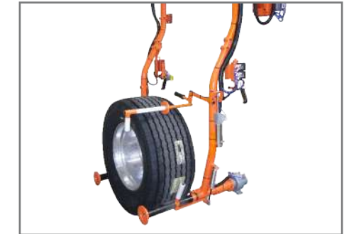
Large Tire Install Nesting style fixture mounted from a Knight Servo Arm. Pneumatic rollers allow for the operator to power rotate tire to the lugs on vehicle.
