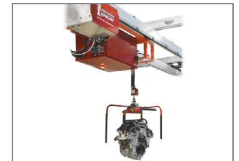
Engine Transfer Hook style end effector operated by a XYZ Servo Hoist and Tractor system. System assists operator in moving the large engine from the line conveyor to the dunnage.
