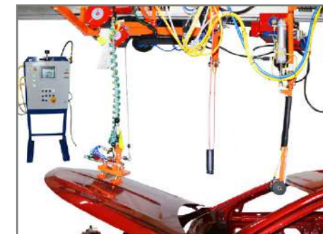
Front Hood Open Vacuum style end effector operated by a programmable PLC system that controls the Air Balancer and Electric VFD Tractor that automatically attaches and raises the hood to operating level.
