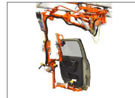
Doors-On Install Servo Actuator, clamp style end effector operated by a programmable PLC system that controls the precise position and angle of the door for installation onto the vehicle.
