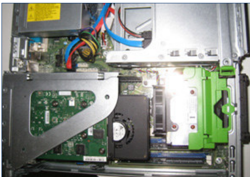
» A full-height professional graphics card, the NVIDIA Quadro® M2000, is shown inside the compact FUJITSU CELSIUS J550 SFF workstation.
