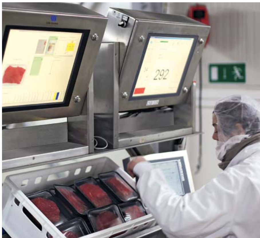
At the CSB-Racks, the pickers can easily see which order is currently being processed, which products and quantities belong to which order, and which label needs to be attached
