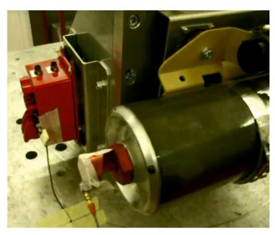
Individual assemblies of the systems have been subjected to a battery of tests both in-house and externally during our work with the MOD including; low and high temperature extremes, drop testing for function after an IED blast, battle field simulations, EMC and vibration testing. Systems have been constantly fielded in Iraq and Afghanistan since 2009 providing assurance that laboratory testing translates to reality.
