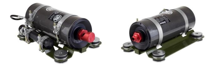
The core of the system; used on Foxhound and Warrior platforms and in-process of being specified on several other UK MOD platforms. The compression discharge cylinder, which can be mounted in any orientation, can be filled with Novec 1230 clean agent suppressant and uses a remote cartridge to provide super-pressurisation only when required at point of use.
