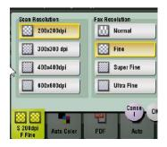
**RESOLUTION:** The option to change the DPI (dots per inch) on scans. Basic text documents are fine at 200x200, would only move up higher for high-quality photos. Keep in mind that the higher the DPI (or the fineness on faxes), the bigger the file.
