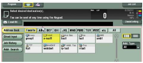
Select the destination from the address book, or to type in choose "direct input." Multiple destinations can be selected at once. A shortcut to dial for fax would be to simply hit the "10-Key" button, which brings up the keypad.
