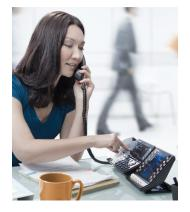
The ShoreTel BB424 gives operators 24 programmable buttons and four page keys, to handle up to 96 lines on a single box or distributed over two.
