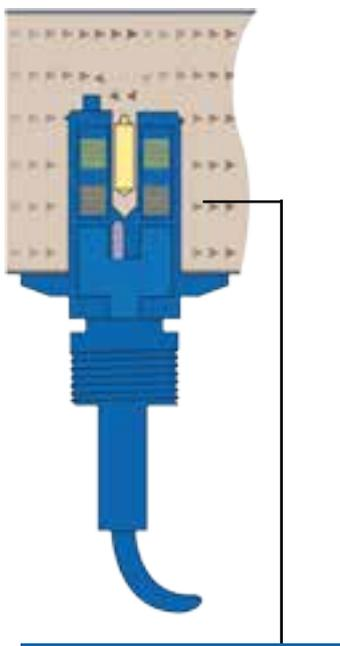
The robust Cambridge Viscosity oscillating piston system can measure a wide range of samples, including asphalt, lubrication oils, and heavy fuel oils, as well as handle any process upsets without damage to the system.
