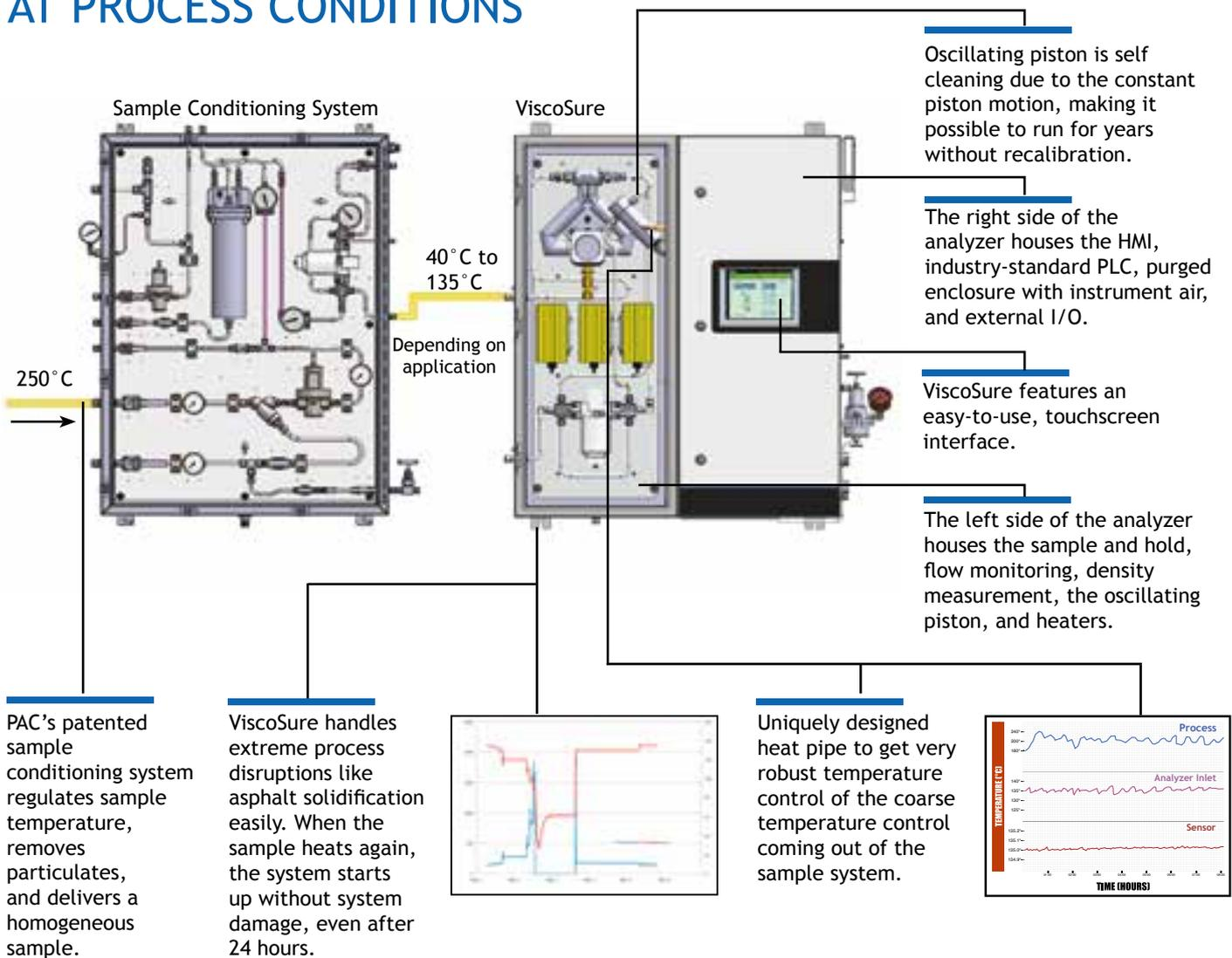
PAC's patented sample conditioning system regulates sample temperature, removes particulates, and delivers a homogeneous sample.
