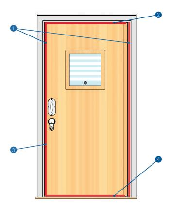
Seal runs the length of the top edge, providing maximum safety
