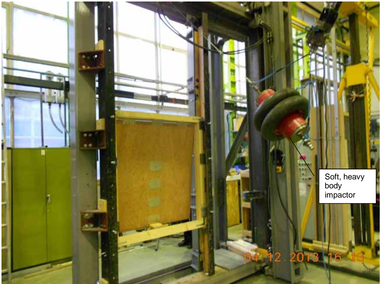
Figure A5. Typical test set-up for impact testing
