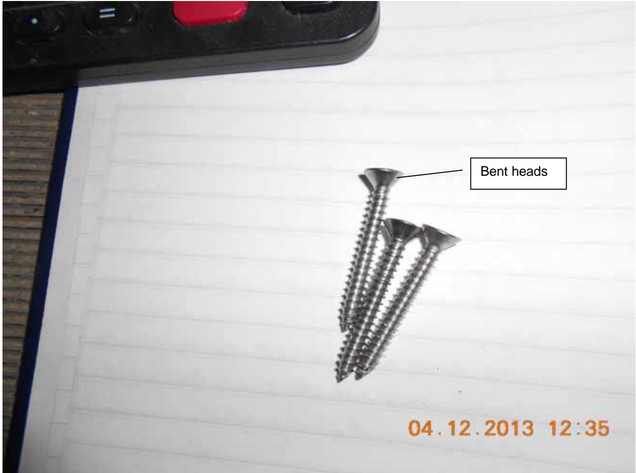
Figure A6. Damage to fixings caused by load testing
