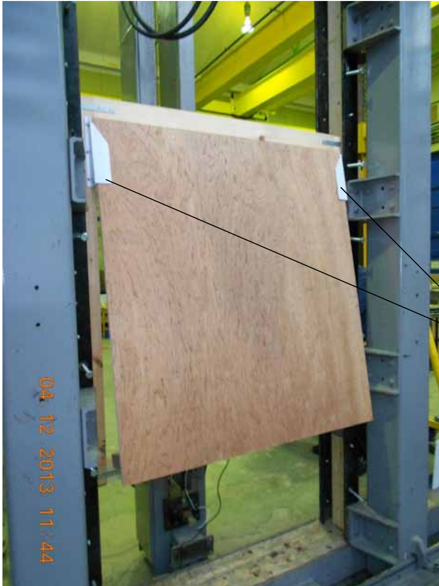
Figure A3. Typical test set-up showing 8WR 225 mm long restrictors
