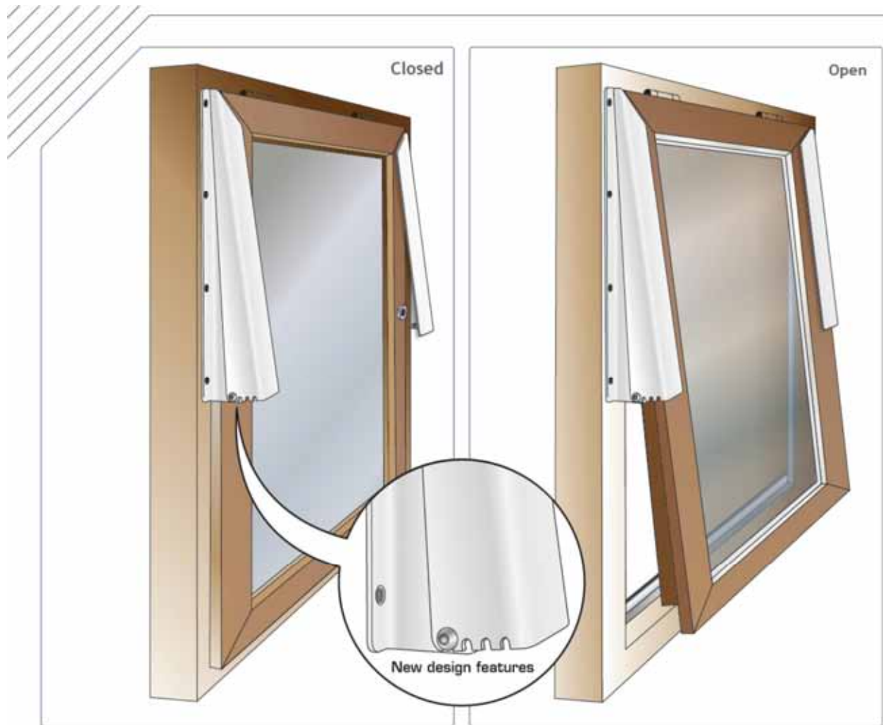
Figure A1. Manufacturer's diagram of 8WR Primera Ltd window restrictors showing pre-set details and general fixing arrangement on a top hung window
