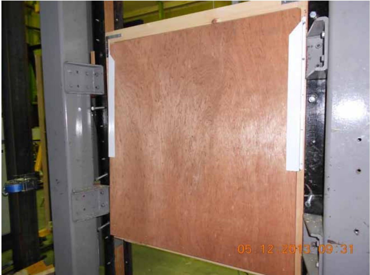
Figure A4. Typical test set-up showing 8WR 650 mm long restrictors
