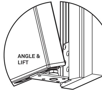
7. If gap between bottom pivot plate and door exceeds 9mm, a long stem bearing **MUST** be used. See page 11
