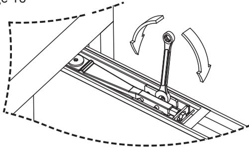
14. Anti-ligature washers MUST be fitted to closer cover plate before installing. See page 17
