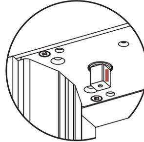
6. To preserve bottom bearing, **LIFT** the door on and off - **AVOID** excessive door angle. See page 12
