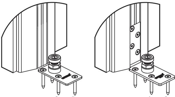
3. Bearing stem lock nut **MUST** be tightened after height adjustment. See page 10
