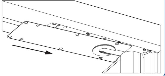
11. Top strap cover plate must be pre-fitted with intumescent strips and secured with 2no. fixings supplied. See page 15
