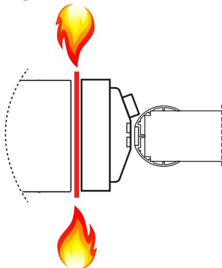
The firestopping requirements between the back of the frame and wall are dependant on the gap size between the substrates. The below information provides the requirements based upon the gap sizes.
