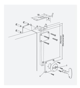
Designed for the most extreme environments, the Rhino Bolt's extended mortice lock bolt secures the slave-leaf to the door frame. Steel deadbolts, high-impact strike plates, bolt-through reinforcing plates and anti-tamper fixings are also used.
