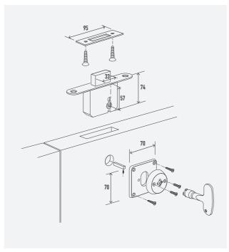
When securing slave-leaf doors is a priority over impact resistance, the Junior Rhino is suitable. The mortice lock is located at the top or bottom edge – or both – and locks the slave-leaf to the floor or door frame. Plus no specialist equipment is required, making it convenient to retrofit onsite.
