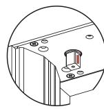
6. To preserve bottom bearing, LIFT the door on and off - AVOID excessive door angle. See page 12
