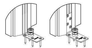
3. Bearing stem lock nut MUST be tightened after height adjustment. See page 10
