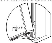
7. If gap between bottom pivot plate and door exceeds 9mm, a long stem bearing MUST be used. See page 11
