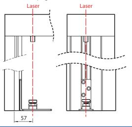
2. Use ALL Floor plate or L-bracket fixings supplied. The L-bracket MUST be fixed to the frame AND floor. See page 9
